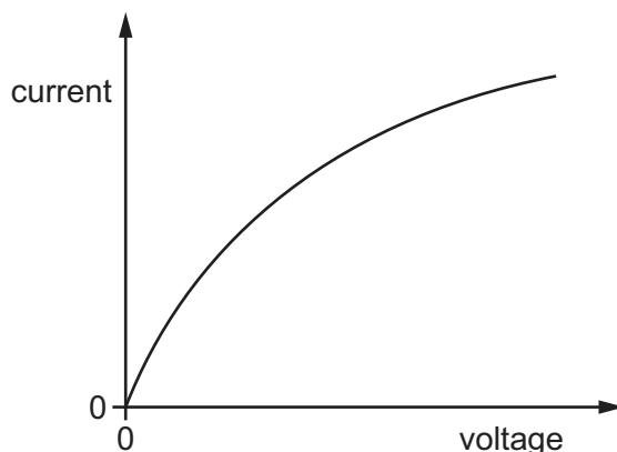
As the current increases, what happens to the temperature of the lamp filament and what happens to the resistance of the lamp filament?
