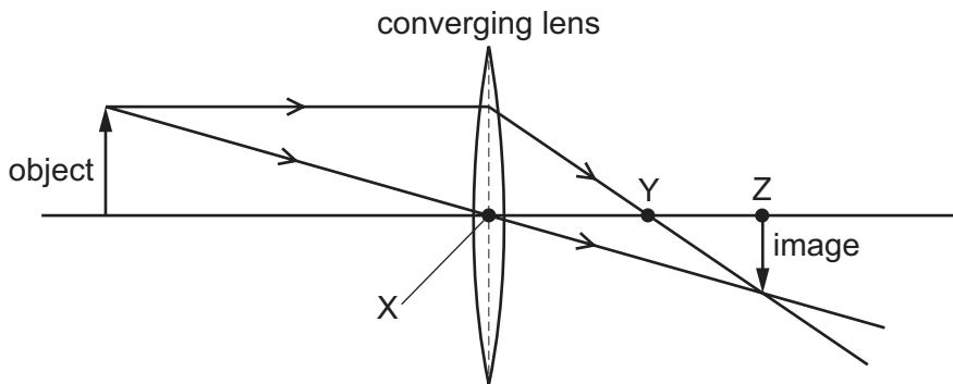
Which labelled point is a principal focus of the lens and which distance is the focal length?
